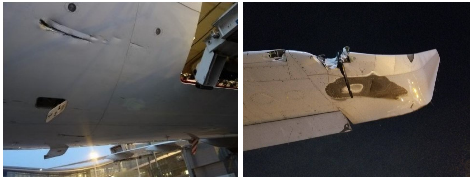
(a) Qatar Airways plane with damage to fuselage. Source: [8] (b) American Airlines plane with runway marker embedded in wing. Source: [5]
