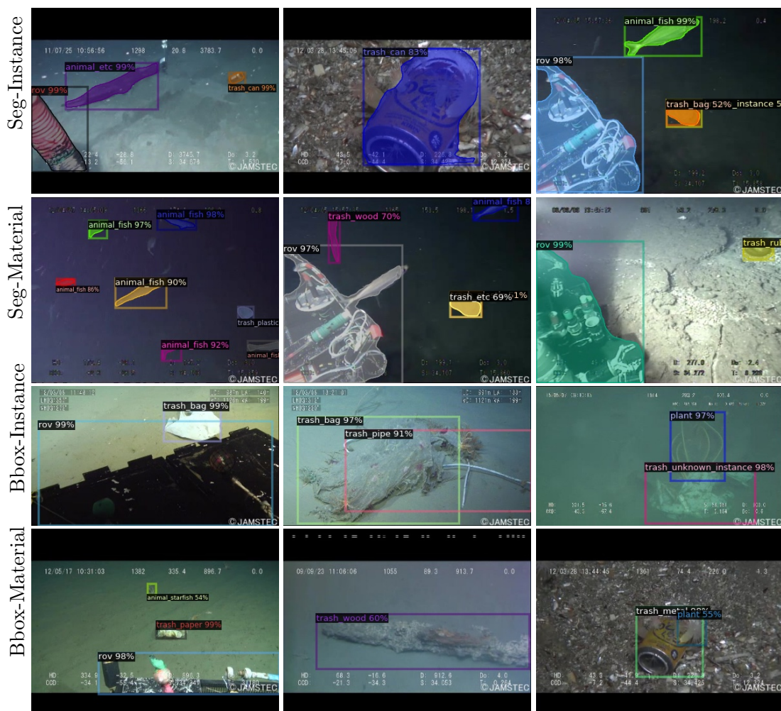
Figure 3.3: Sampled results for object detection and image segmentation for both versions of the TrashCan dataset.
