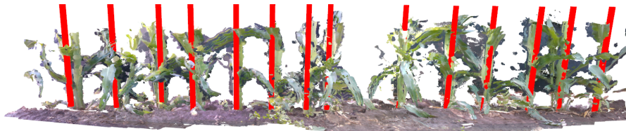
Figure B.4: The reconstructed point cloud of a corn row and the estimated corn stalk position (red cylinders) from ROW SLAM.
