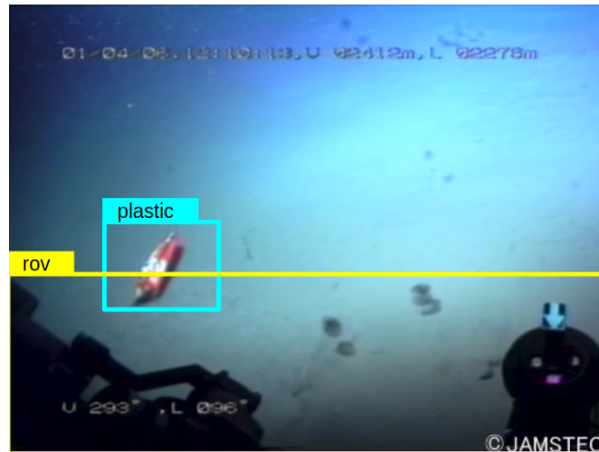
Figure 2.1: An example of a labeled training image showing two classes: the ‘plastic’ class in blue, and the ‘ROV’ class in yellow.
