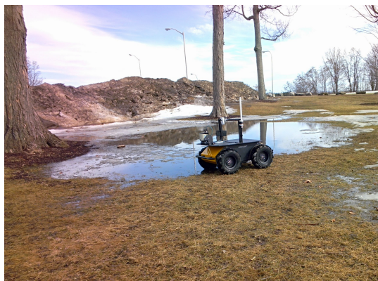
Fig. 1: A Husky AGV robot during a robot field trial. The exploration of large, unstructured outdoors environments is a likely scenario for adaptable natural language communication in human-robot teams.
